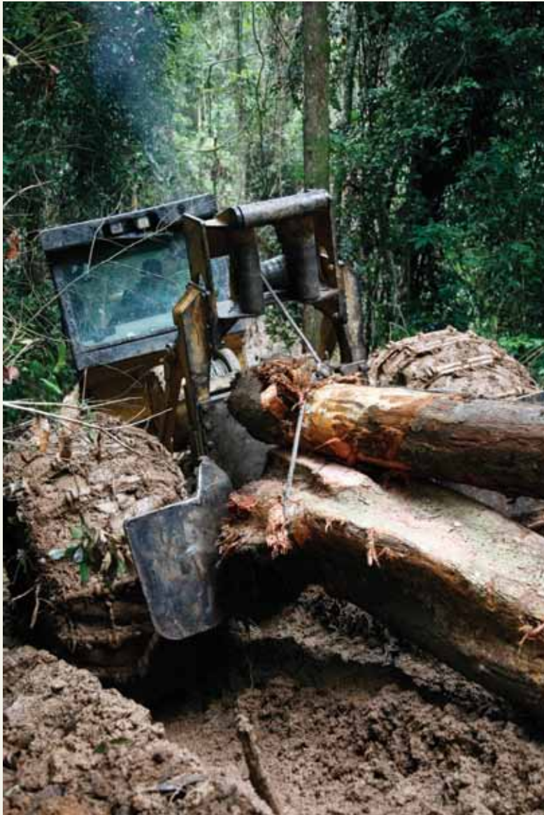
A 'track skidder' at work in the forest. The skidder pulls the tree from the production site to the road where it will be loaded onto trucks. The 'track skidder' has a narrow shovel, to reduce the damage to the forest by working on narrow trails. This is an FSC requirement. Tropical rainforests, western Ghana.
