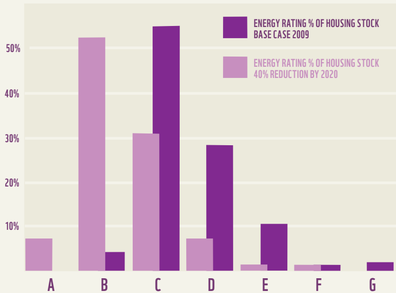
FIGURE 2.1 INDICATIVE ENERGY RATINGS FOR THE HOUSING STOCK AS A WHOLE IN 2020 UNDER THE 40% BY 2020 SCENARIO APPLIED TO WHOLE HOUSING STOCK
