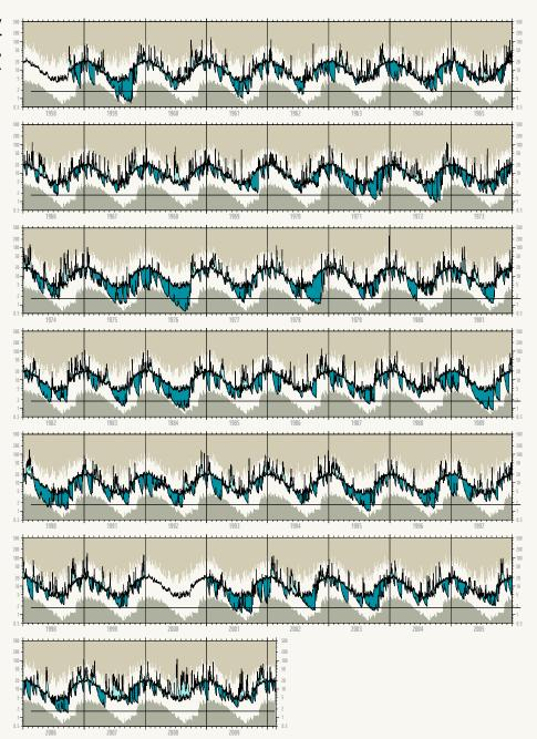
The areas shaded in dark blue show flow periods below the long term mean flow. The areas shaded in light blue show flow periods above the long term mean flow. Note the use of the logarithmic scale on the vertical axis. The line across the hydrograph represents the Q95, or flow exceeded in the river for 95% of the time, an indication of the level below which the environmental risk from abstraction increases.
